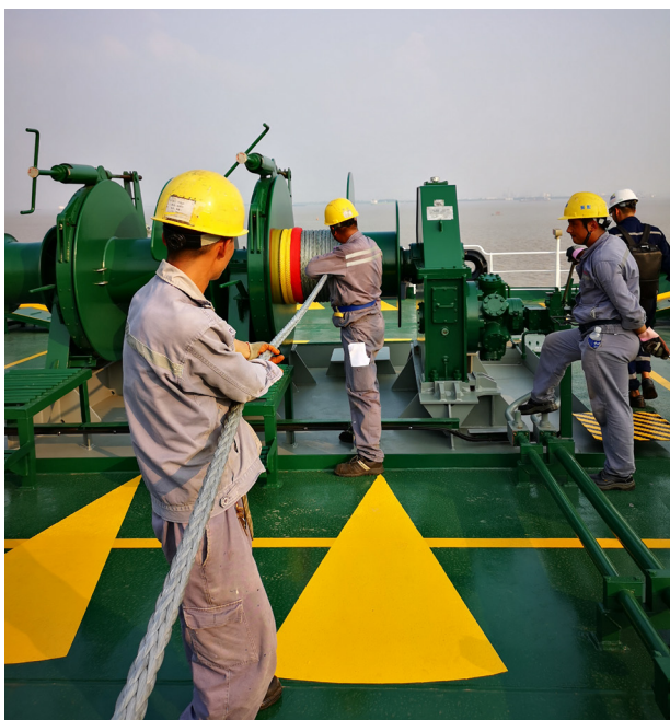
Figure 1. Timm™ Acera Amundsen installed on a new tanker vessel, with focus on correct installation. The two first layers on the winch need to be lightly tensioned, for easy installation of the following rope layers.
