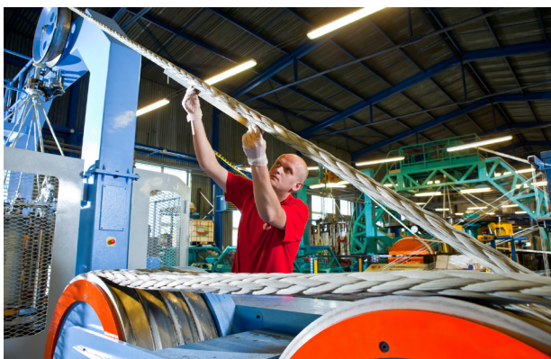
Figure 2. During production, it is important to do quality checks to make sure that a high realisation factor is kept. The realisation factor is an important part of identifying how much strength of the original fibre is kept in the final rope design.
