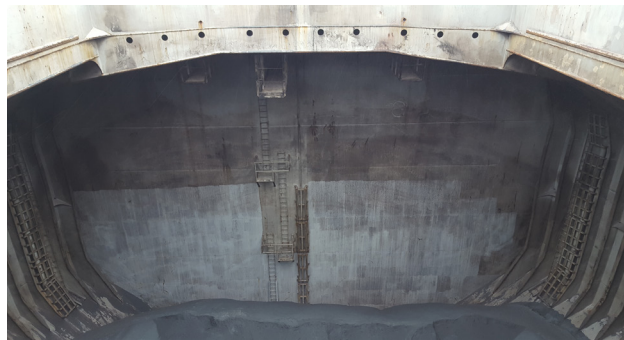
Figure 3. Newer paint coatings prevent strong adhesion of cargo particles vs older paint coatings. Older coating: upper part; newer coating: lower part. An additional temporary barrier coating enhances efficiency by allowing even less cargo to stick to the surface after washing the holds.
